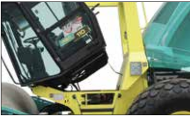
Tilting cabin for safe and easy maintenance and service
